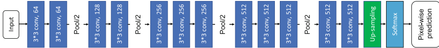
Fig. 4.7 The modified architecture of VGG16 for semantic segmentation. The number after “conv” represents the number of filters (e.g., “3 × 3 conv, 64” represents 64 convolutional filters of a 3 × 3 dimension)
