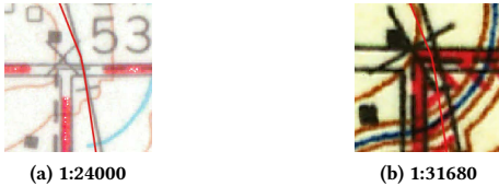
Figure 3: An example of the railroad (the black line with crosses) in different scales (the red line is the vector data)
