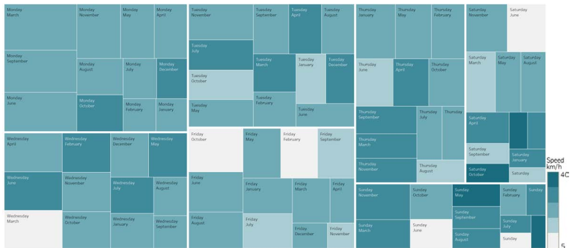
Figure 3: A time cartogram representing the temporal distribution of vehicle movements and their median speed on Sankt Peders Gade. The big rectangles represent weekdays and small rectangles inside 12 months. The size of the rectangle indicates the amount of the trips: min 7 – 14 and max 45 – 65 per weekday over the months. The color saturation of the rectangles represents median speed. The darker the saturation the higher the median speed and vice versa.
